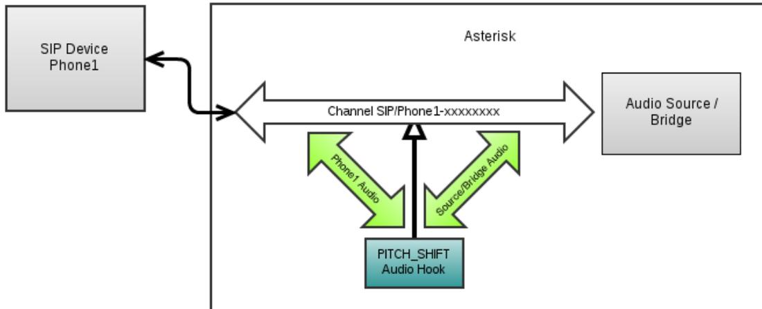
In this simple example, a SIP phone has dialed into Asterisk and its channel has invoked a function (`pitch_shift`) which has been set to cause all audio sent and received to have its pitch shifted higher (i.e. if the audio is voice, the voices will sound squeaky sort of like obnoxious cartoon chipmunks). The following dialplan provides a more concrete usage:
