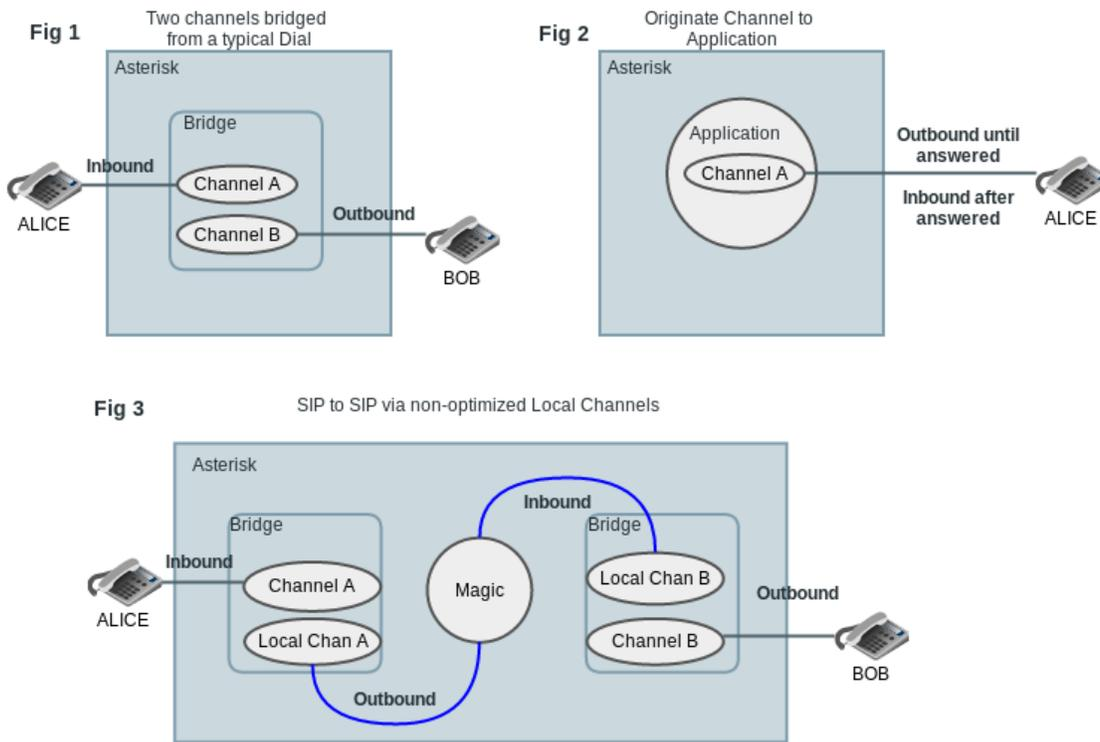
The figures have been kept somewhat generic and should apply to most channel types. Each figure shows the final state of the call, rather than a sequence of events.
