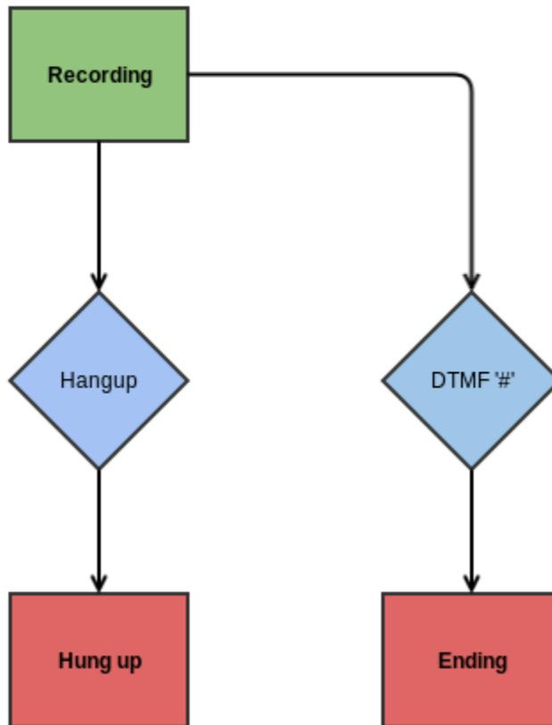
Notice that even though DTMF '#' and a caller hangup result in the same end result that there are two separate states that are transitioned into. This is because our code needs to behave differently at the end of a voice mail call based on whether the channel has been hung up or not. In short, the "Ending" state in the diagram will forcibly hang up the channel, whereas the "Hung up" state does not need to do so.
