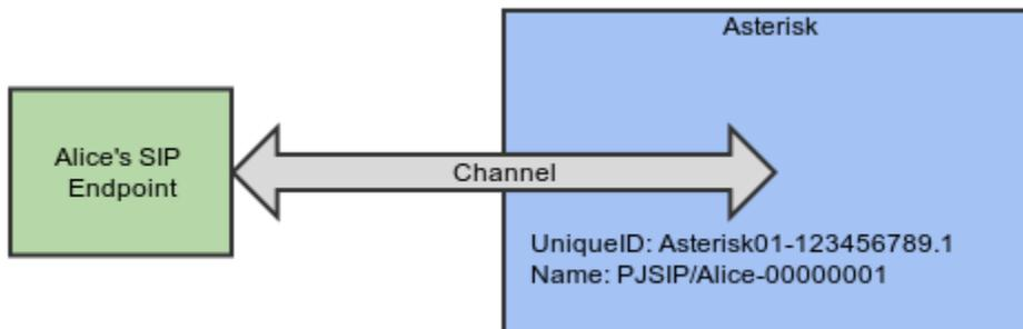
In the above diagram, Alice's SIP device has called into Asterisk, and Asterisk has assigned the resulting channel a UniqueID of **Asterisk01-123456789.1**, while the PJSIP channel driver has assigned a name of **PJSIP/Alice-00000001**. In order to manipulate this channel, ARI operations would use the UniqueID **Asterisk01-123456789.1** as the handle to the channel.
