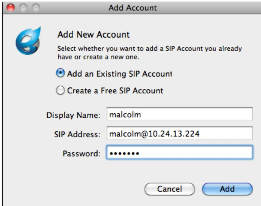
Then, we need to modify the Account Preferences, and under the SIP Settings, we need to set the outbound proxy to connect to the TLS port and transport type on our Asterisk server. In this case, there's an Asterisk server running on port 5061 on host 10.24.13.224.
