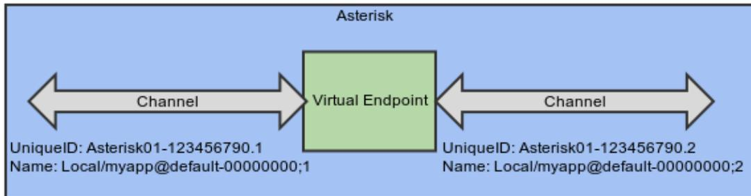
In the above diagram, ARI has created a Local channel, `Local/myapp@default`. As a result, Asterisk has created a pair of Local channels with the UniqueIDs of **Asterisk01-123456790.1** and **Asterisk01-123456790.2**. The names of the Local channel halves are **Local/myapp@default-00000000;1** and **Local/myapp@default-00000000;2** - where the ;1 and ;2 denote the two halves of the Local channel.
